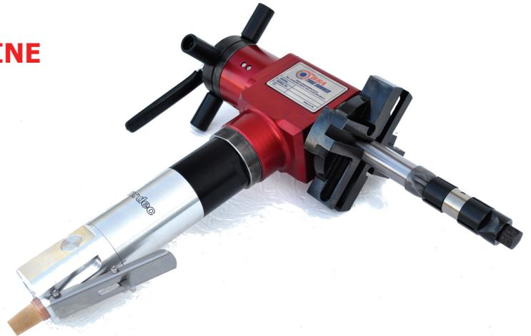
**The Thunderbolt machine is a lightweight, High Power tube-prepping machine, designed to bevel, face and counterbore most types of tube and pipe work.**
