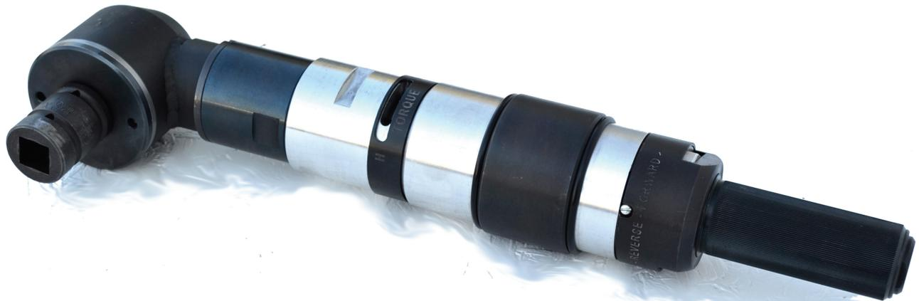
**The Vortex** is a right angle pneumatic torque controlled motor designed for the expansion of Boiler tubes in Steam and Mud Drums, Fire Tube Boilers and similar equipment.
