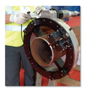
A series of low clearance, split frame, pipe cutting and bevelling machines.
